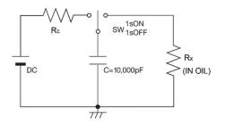
Apply 10 pulses with the voltage listed in the table above to the resistor, the change of the resistance shall be within the requirement range as compared with the value before the load.
